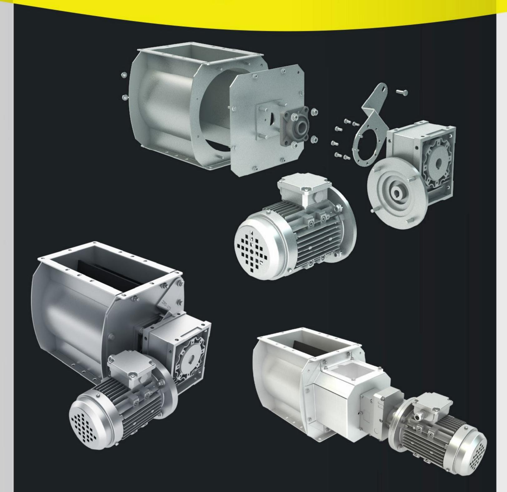
The IST series valves are made of sheet metal of steel welded and subsequently galvanized. These valves are provided of rotors with trated rubber blades easy to replace, which can be optionally supplied also in vulcollan if you need to dose hot products.
